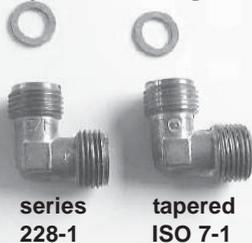
**Caution:** according to the regulations in force in certain countries (see gas table page 26, it is compulsory to replace the cylindrical fitting production mounted on the cooker with a tapered fitting\* supplied with the unit.
